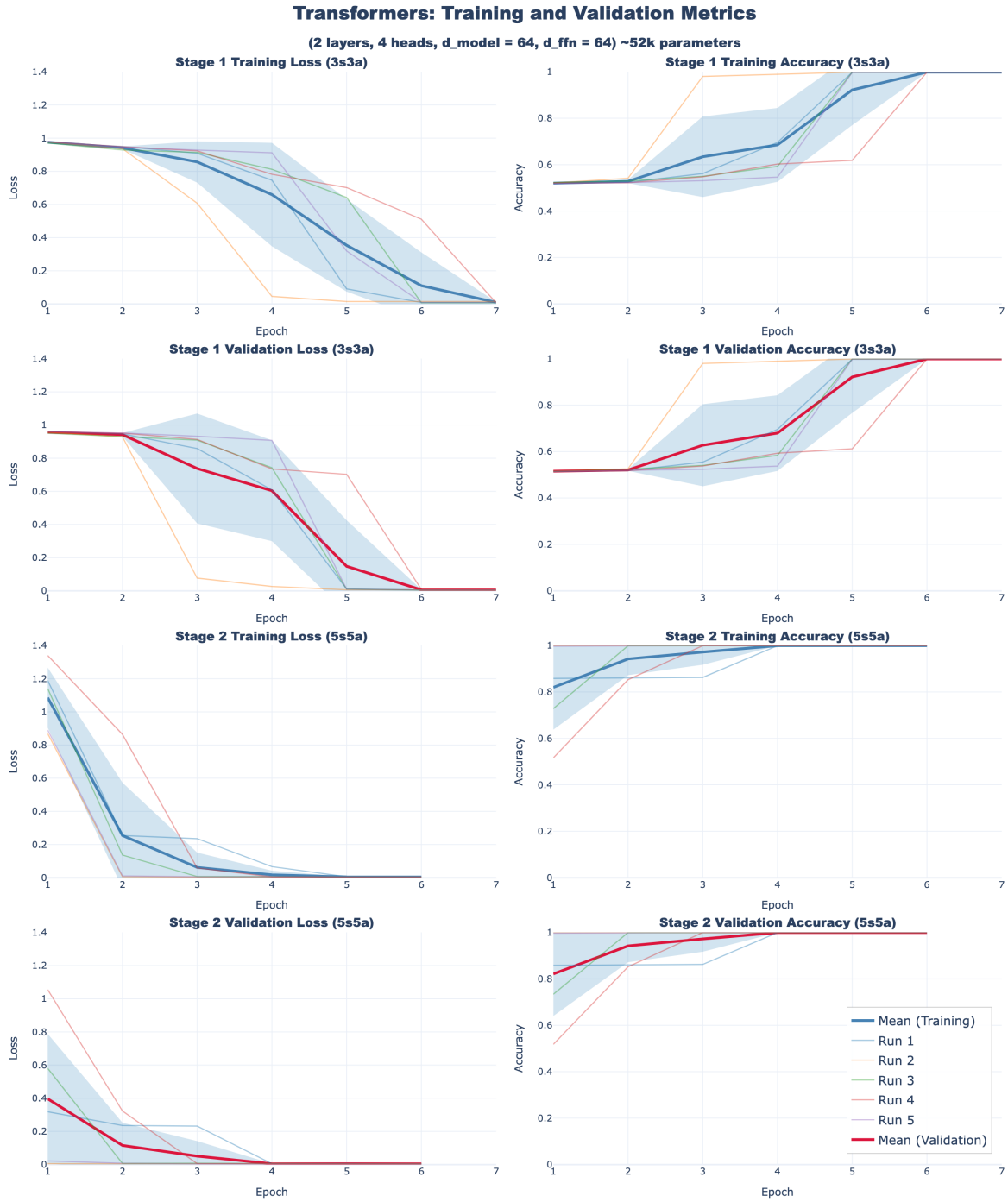
Figure 6: Transformer Training and Validation. Training dynamics showing the necessity of curriculum learning and the “phase transition” phenomenon.
